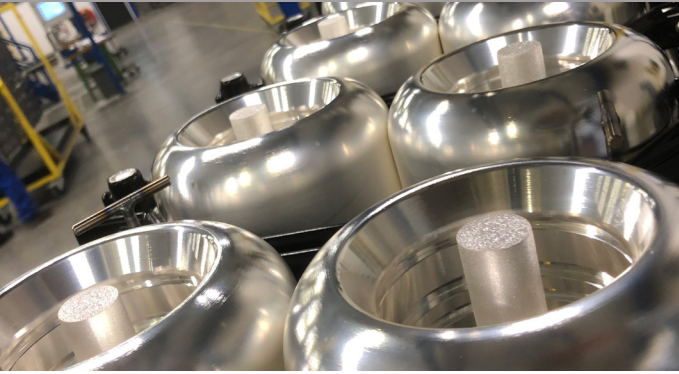
Silver plating of internal diameters with internal anode
