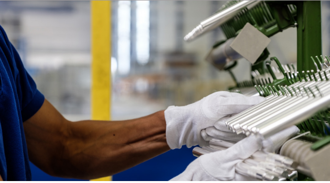
Silver plating on a dynamic rotating rack
